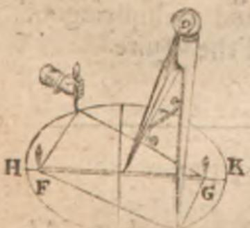
*G.H*, or *F.K*, then if you take a Compasse which may have one foot lower than another, with a spring between his legges: and placing one foot of this Compasse in the Centre of the Ovall, and guiding the threed by the other foot of the Compasses, and so carrying it about: the spring will help to describe and draw the Ovall forme. But in stead of the Compasses it may be done with ones hand only, as in the figure may appeare.
