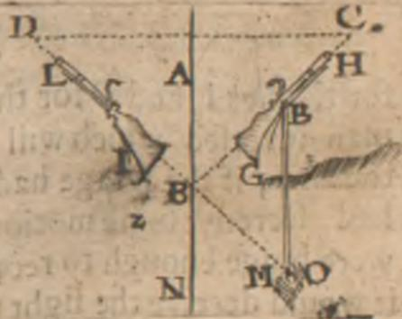
which suppose at  $L$ , so shall it be truly placed; and giving fire to the Musket, it shall not faile to strike the said mark at  $C$ .
