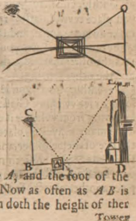
Tower  $E$   $D$  contain the distance from your eye to the foot, *viz.*  $C$   $B$  for the Triangles  $A, B, C$ , and  $A, D, E$ , are equal Triangles: therefore as  $B A$ . to  $A D$ , so  $C B$ , to  $E D$ , or alternately as  $B A$ . to  $B C$ , so  $A D$ .to  $D E$ .
