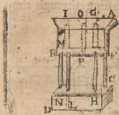
is to say, to make an opening to the cover of the vessell *A B*, & let it have a little mouth as a Trumpet: to that end to receive the water. Then there must further be added a very smal Pipe which may passe
