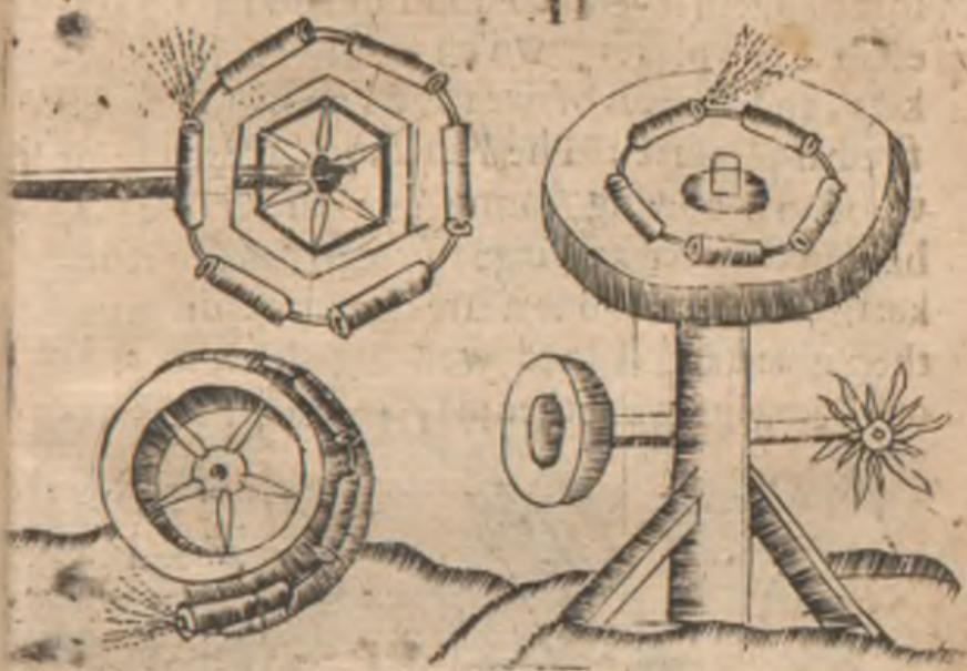
*D*, that *C*; and that will fire the Rocket at *A*; then immediatly the wheel will begin to move, and represent unto the spectators a Circle of changeable fire, and if pots of fire be tied to it, you will have fine sport in the turning of the wheele and casting out of the Serpents.
