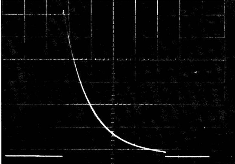
FIG. 3. *Waveshape spikes sharply up to about 3.2 volts and subsides rapidly, with 90% of spike over in 2 msec., although voltage does not return to zero for about 8 msec. (abscissa calibration: 2 msec. per square; ordinate calibration; 0.5 volt per square).*
