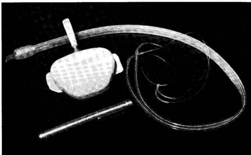
FIG. 1. Current pacemaker model has Silastic case; strip of Silastic-impregnated Dacron mesh facilitates suturing of case to anterior rectus sheath. Note the slip fit for helicable twin electrodes and magnet for external rate adjustment.
