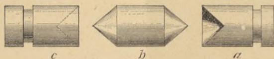
FIG. 1.—The carbons, twice the natural size: a showing countersunk section of c ; b showing double cone.
